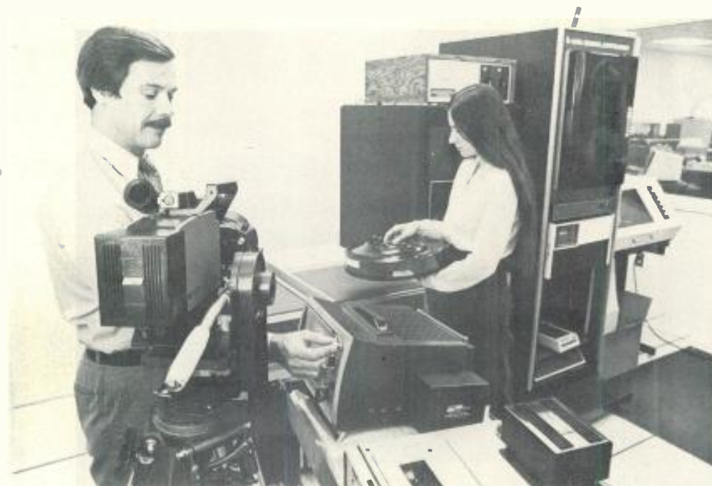
Anton/Bauer's silver zinc batteries being computer-tested while in use.
