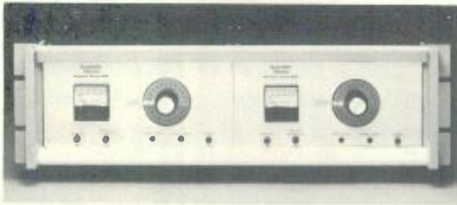
An automatic local ad inserter, such as the C-150 from Microtime, originally designed for cable TV, could find applications in conjunction with nationally networked radio programming.
