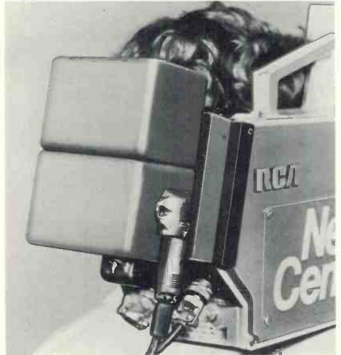
The on-board nicad by Alexander is hooked to an RCA video camera.
